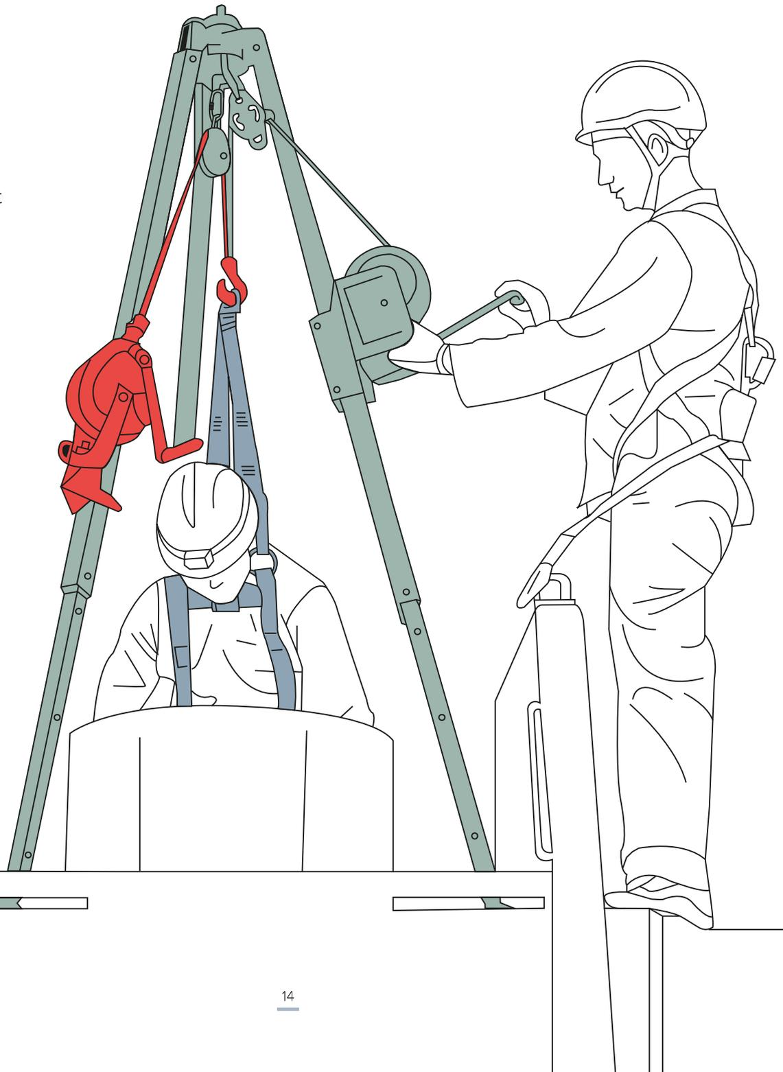
Davit arms and tripods are used to enhance the safety whilst entering, leaving, and accessing confined spaces. Rescue missions can be performed effectively by winching an injured person in a harness to safety. Fallprotecs's davits and tripods made in AISI304 has been specially developed for mobile use in conjunction with the RopeClimber hoist, HRA Rescue device and winches.
