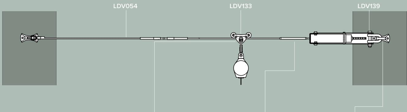
The LDV133 is the proper glider when the connecting device is a self-retractable fall arrester that weighs 10 kg or less. The glider passes smoothly over the intermediate anchors. The end user can move freely along the lifeline without disconnecting and hands-free to operate with tools. If the user is less than 3 m below the life line, a 2 m absorbing lanyard, connects the user to the captive glider LDV060.
