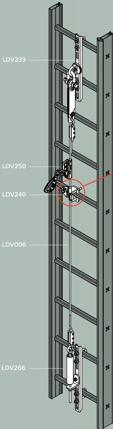
Intermediate anchors clipped on the cable, can easily be retrofitted on a lifeline. Span between anchors 10m (32'8")
