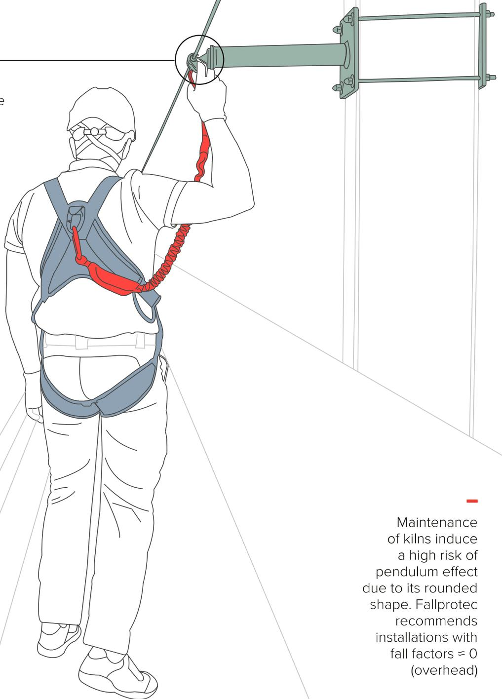
Maintenance of kilns induce a high risk of pendulum effect due to its rounded shape. Fallprotec recommends installations with fall factors  $\approx 0$  (overhead)
