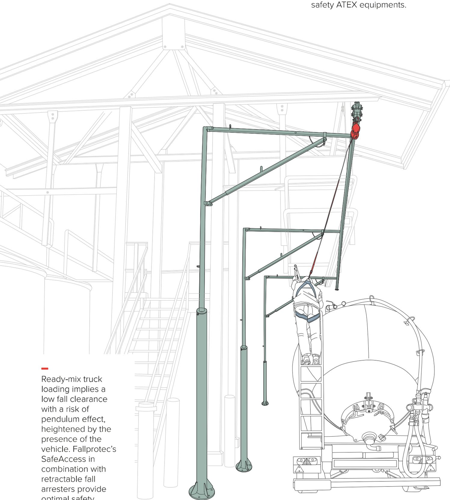
Ready-mix truck loading implies a low fall clearance with a risk of pendulum effect, heightened by the presence of the vehicle. Fallprotec's SafeAccess in combination with retractable fall arresters provide optimal safety.
