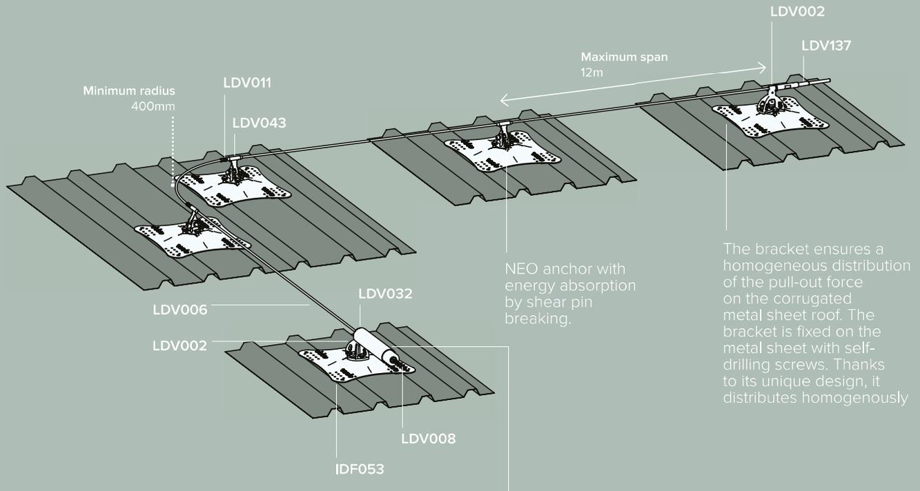
The energy absorber is a key component of an engineered cable lifeline. It reduces the forces transmitted to the host structure. Combined with the intermediate anchor LDV043 with integrated shock absorber, it enables the installation of the cable lifeline on a great variety of fragile roofs and structures. The energy absorber has 4 functions: energy absorption in case of a fall, indicator of the tension in the line, upkeep of the tension in the line and indicator of a fall.
