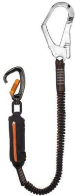
**Elastic lanyard 2m, energy absorber fitted with pivoting carabiner and hook 60mm opening**
