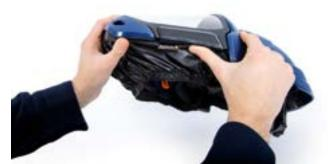
**7.4** Press the face seal all around the visor. Make sure that the face seal pins is fixed in the visor. Secure the face seal hooks into the head harness.
