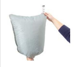
2.2 Place the head-top in the flow meter and start the fan unit. Grip the bag to seal around the breathing hose. Grip the flow meter tube with the other hand, the tube will point upwards from the bag
