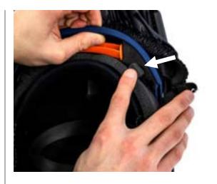
**8.3** Fit the new forehead seal. Press down the tabs of the forehead seal in the socket on the face shield.
