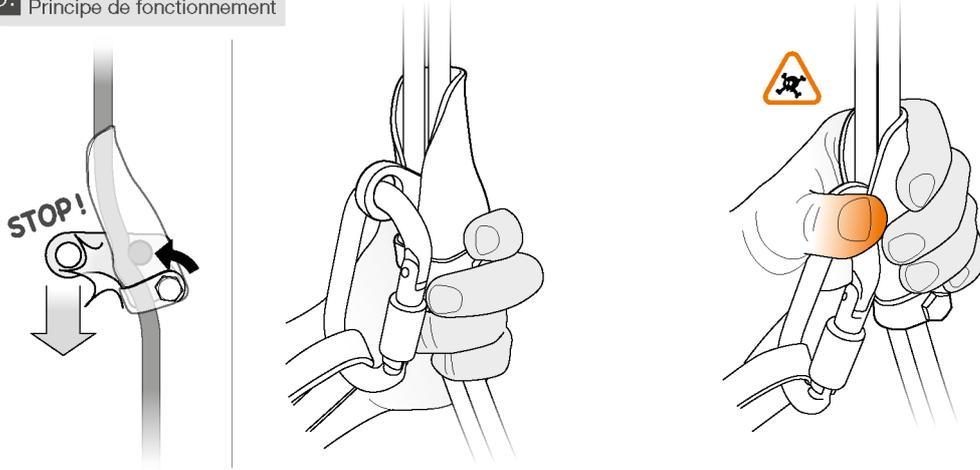
6. Installing the SHUNT
