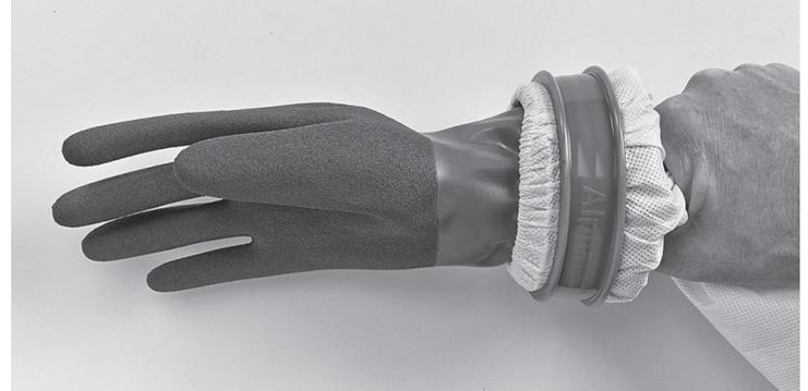
**Step 6** - Hold the sleeve of the coverall as shown and check there are minimal creases on the sleeve end and gently push the AlphaTec® green collar up the sleeve so that the sleeve cuff is exposed and the collar is beginning to tighten on the inner glove cone.
